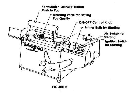
5. After setting the fog quality, the fog may be started and stopped by pressing and releasing the FORMULATION ON-0FF BUTTON.
