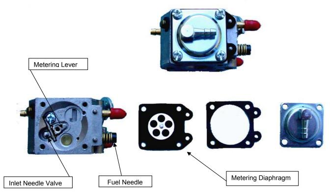
**Carburetor – Metering Chamber Side**
