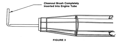
2. Continue rotating the tool in the same direction and pull back and remove the brush from the tube.
