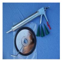
For applications using 10oz tubes a standard size caulking gun will be required.
