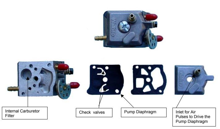
**Carburetor – Pump Chamber Side**
