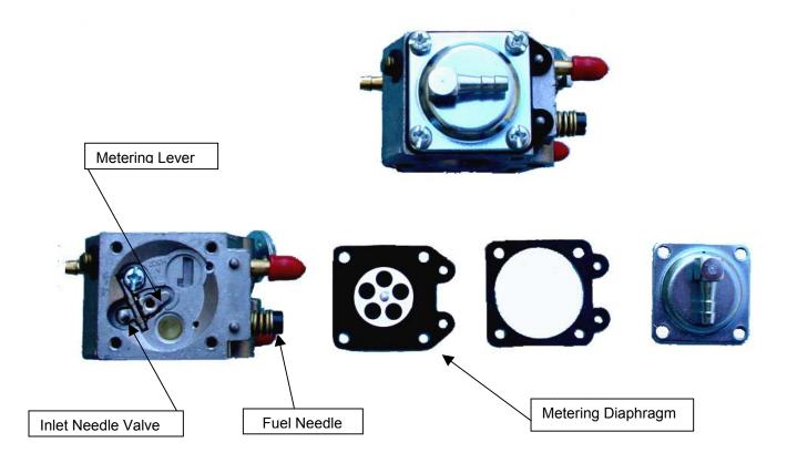
**Carburetor – Metering Chamber Side**
