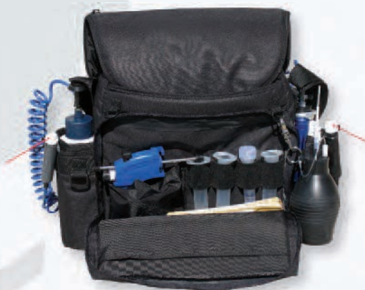
Kit—including ADU, AccuSpray, Bulb Duster and Low Profile Monitors
