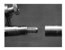
A 3/8 open-end wrench can be used to tighten the packing nut if the valve develops a leak.
