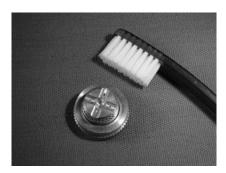
The filter is located between the hose and the valve; loosen the fitting, remove the filter and clean with a toothbrush. This filter keeps dirt out of the valve and nozzle, replace if it is lost.
